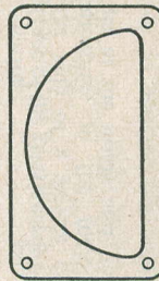
ANOTHER PIECE OF PERSPEX WITH A SEMI-CIRCLE CUT OUT SAME SIZE.
